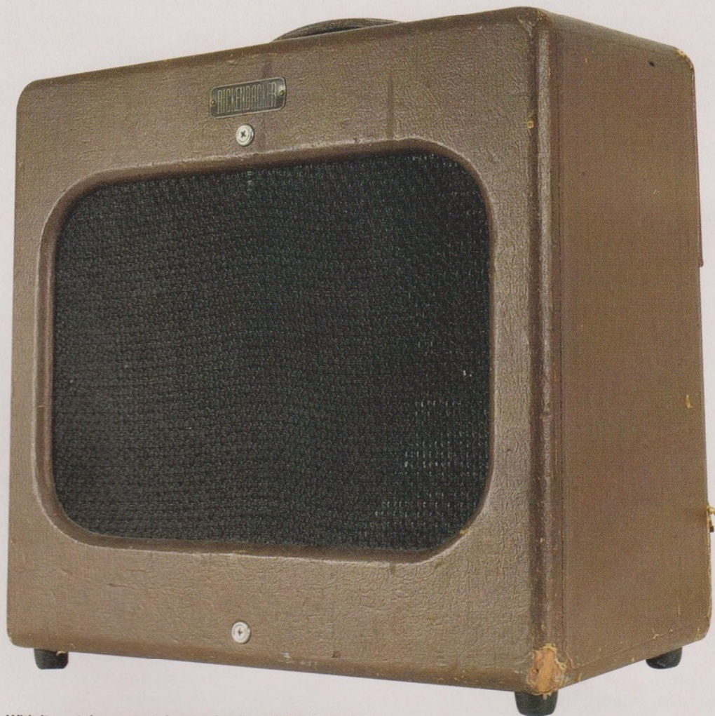
With its octal preamp tubes and pair of 6V6s, the M-11 is very similar to an early tweed Fender Deluxe.
