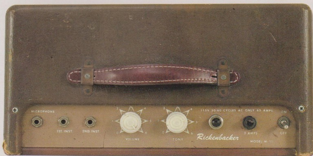
With its octal preamp tubes and pair of 6V6s, the M-11 is very similar to an early tweed Fender Deluxe.
