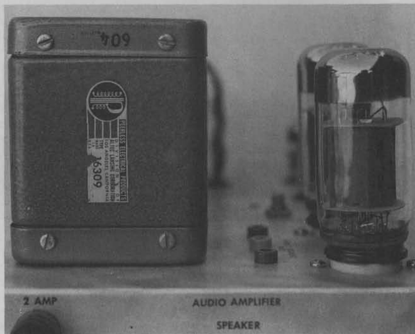
This Peerless output transformer, vintage 1950s, was a hot item in top-quality 20-watt audio amplifiers. Prices then were from $2 to $5; they are now valued from $75 to $150.
