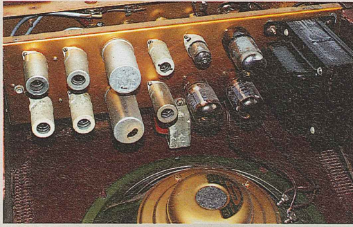
Ten of the 11 tubes in the EchoSonic, on the crowded underside of the chassis, alongside two multi-section capacitor cans and a large power transformer.
